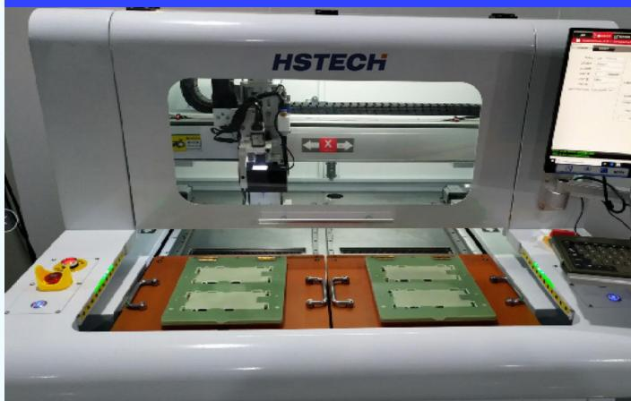
In the twin table working mode, the machine's space and time resources can be fully utilized to achieve efficient production scheduling and improve the machine's utilization rate and production capacity.
